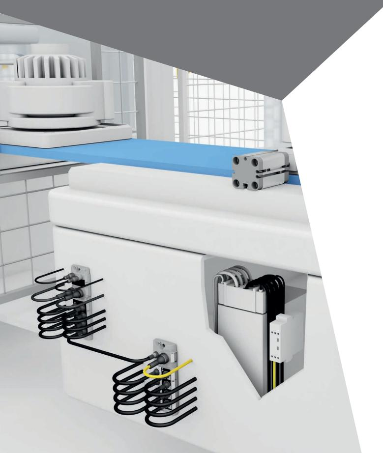
The BNI IOL-355 galvanically isolated sensor/actuator hub offers you an all-in-one solution for connecting both sensors and actuators. With this innovative block you can operate up to eight digital in- and outputs. At the same time, you can safely turn off the actuator segment via its separately switchable safety circuit because the IO-Link I/O hub is divided into two galvanically isolated segments.
